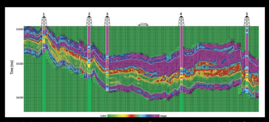
Arbitrary line through an acoustic impedance volume passing through five wells. The acoustic impedance volume as well as a Gamma Ray volume generated using neural networks were used together to generate facies a volume for the Vaca Muerta shale interval, Argentina (Data courtesy: Pan American Energy)
