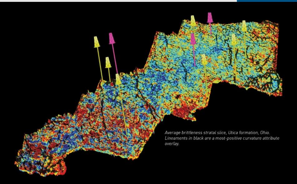
At TGS we seek more meaningful approaches to shale characterization. For example, where appropriate, we describe shale zones in terms of 'fracture toughness', which is measure of resistance to fracture growth. This offers better results in various shale formations across North America, especially where brittleness and stress strain do not always correspond to a typical high Young's modulus and low Poisson's ratio relationship.
