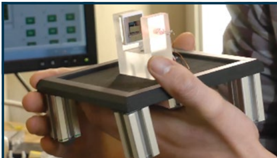
The new gravimeter created by researchers at the University of Glasgow in Scotland's Institute for Gravitational Research uses the same type of micro-electromechanical system (MEMS) used in smartphones' internal accelerometers. Image courtesy of the University of Glasgow.
