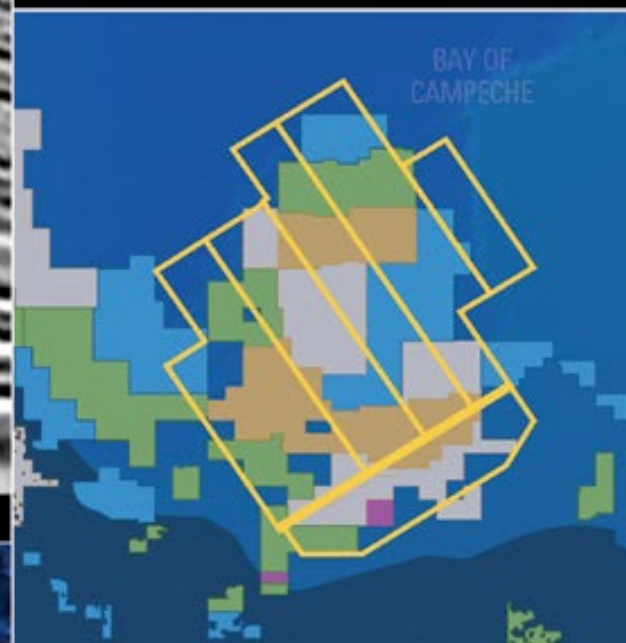
Reverse time migration showing three- and four-way salt body closures.
