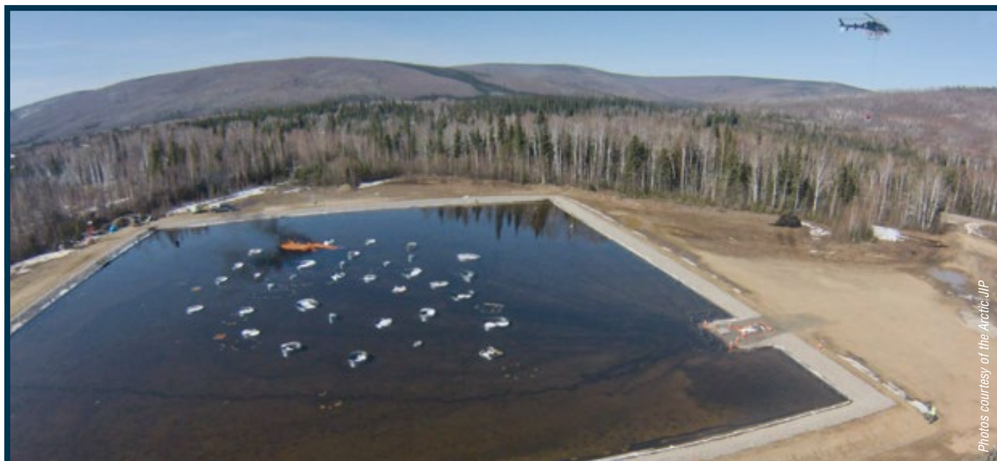
The Arctic JIP experiments with herders and burning in a massive tank at the Poker Flat Research Range.
