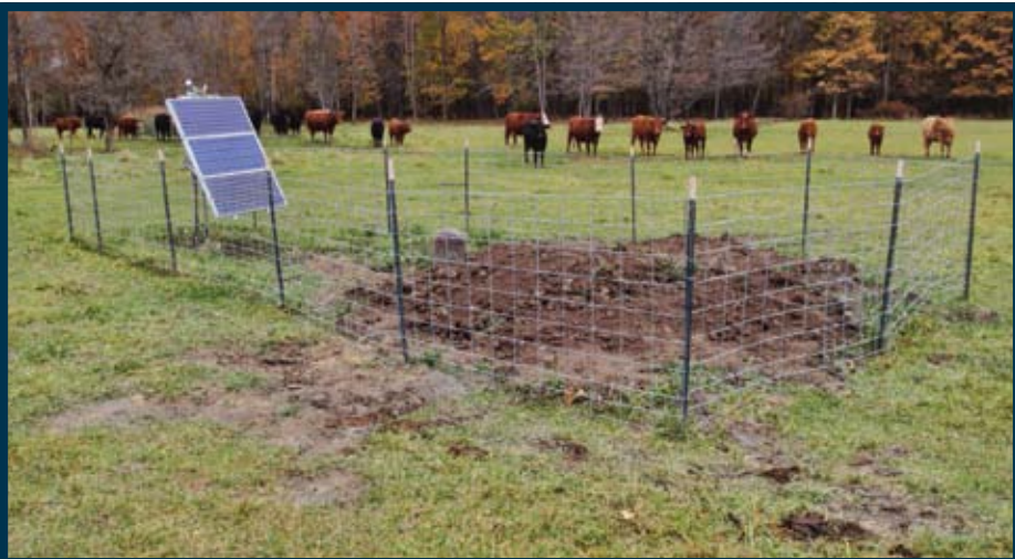
Transportable Array station K50A, near Lake St. Clair in Casco, Mich. The vault is covered with a mound of dirt to provide thermal insulation, and solar panels recharge the batteries that power the station. A high-performance barometer and an infrasound sensor (located between the vault and the solar panels) measure atmospheric conditions.
