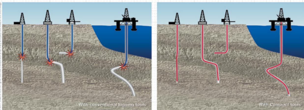
Compact formation evaluation (FE) tools are half the size of most conventional wireline equipment and offer **eleven different conveyance options**. So now you can gain access to more hole sizes and log problematic wells with less risk of getting stuck.
